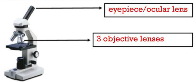
Since compound microscopes have 2 lenses, you must multiply each of the lens magnifications to get the total magnification.
